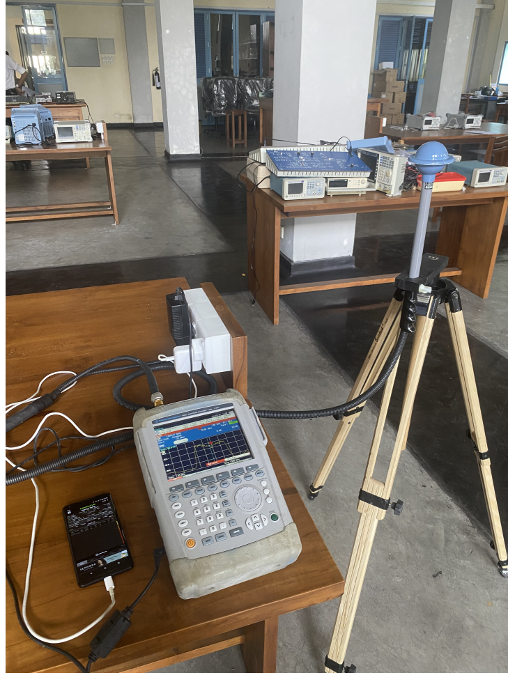
Figure 3.1: Test setup for validating mobile phone reading.
